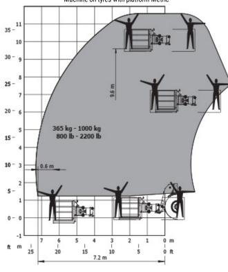
Machine on tyres with platform Metric
